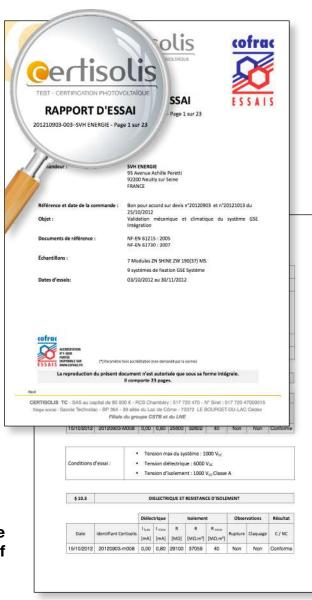
The GSE IN-ROOF SYSTEM subjected to the UV radiation pre-conditioning test **exhibited no visual defect after 15 kWh.m2 of exposure to UV radiation.**
